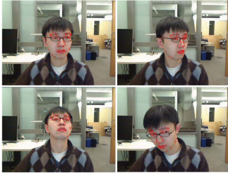
FIG 2: Head tracking using a regular camera.
