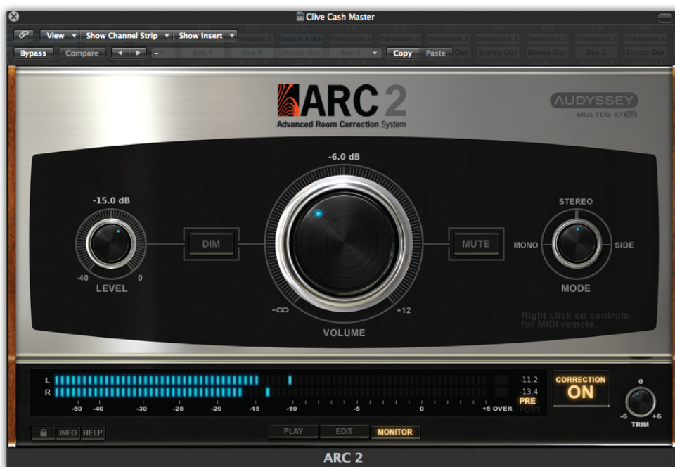
The ARC 2 plug-in's monitor controller page includes Dim, Mute and various stereo options, as well as a MIDI-controllable volume knob.
