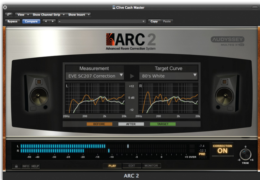
The ARC 2 plug-in lets you select from multiple measured curves — if, for instance, you have several sets of monitors — and apply either a flat response or, as here, a Virtual Monitoring speaker emulation.
