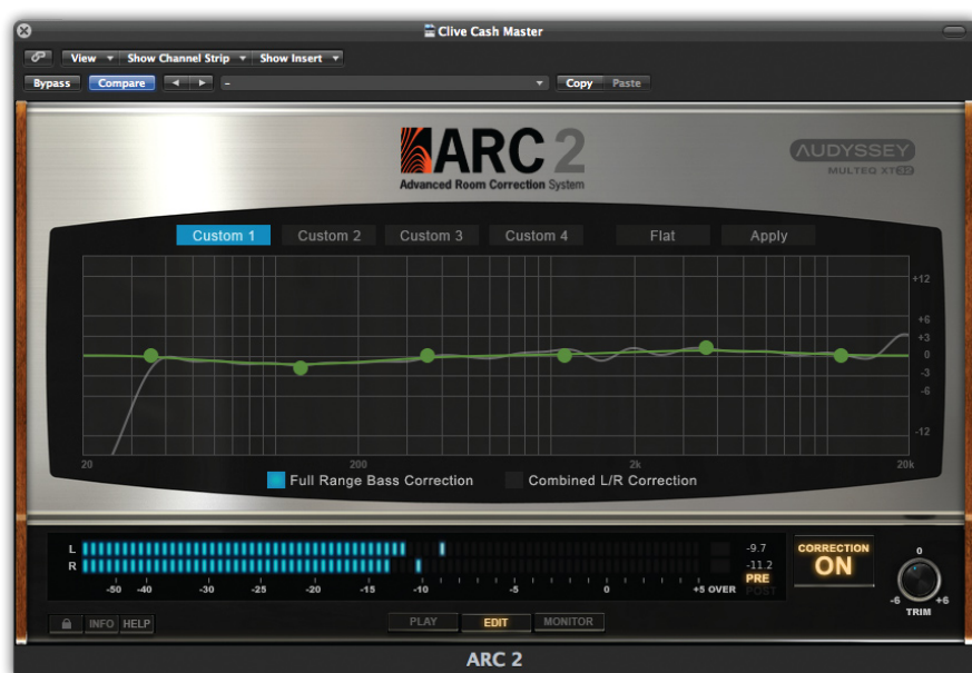
New in version 2 is the option to apply a user-defined EQ curve to the monitor correction.
